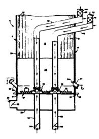
A fluidized bed heat exchanger in which a perforated plate is disposed within a housing for supporting a bed of particulate material. Air is passed through the plate to fluidize the particulate material and a mixture of air and additional particulate material is introduced to said bed and deflected into said bed in a manner to induce diffusion and circulation of the bed materials in the bed.
